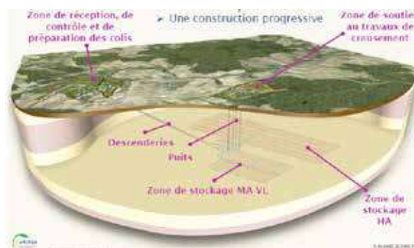
Figure 3 – The CIGEO Storage Project
