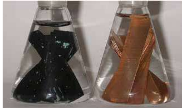
Appearance of copper after 15 years of exposure in distilled water at room temperature. Hydrogen from corrosion can escape from the left container but not from the container to the right. The water volume was equal in the flasks in beginning of the exposure.
